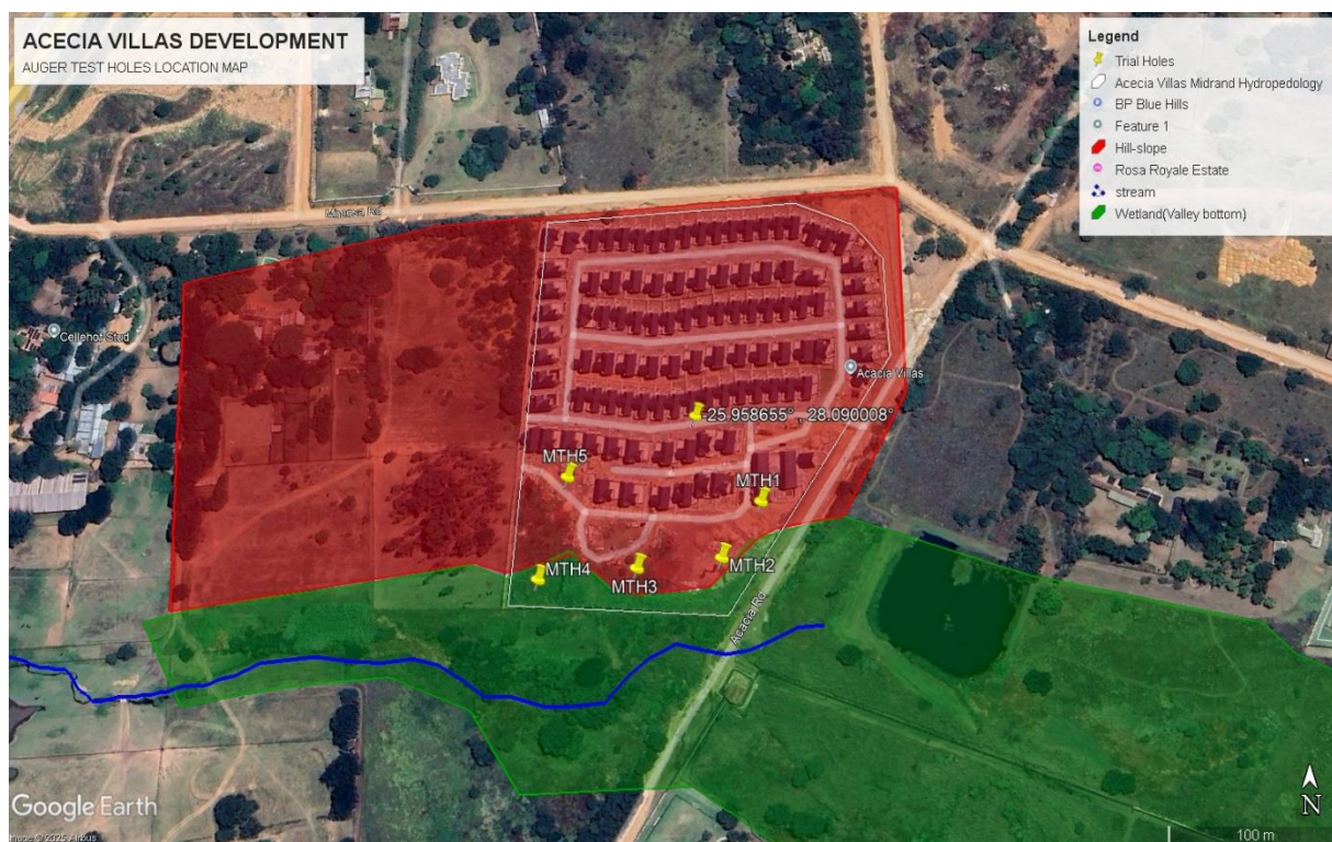
Figure 10: Shows position of test holes in the investigation area.
